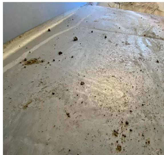
**Photos Above:** K-Floshield® after install shows no signs of wear and maintains original shine and slipperiness. Hang up issues resolved.
