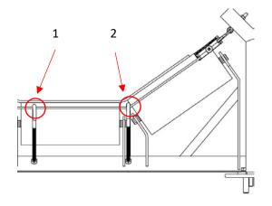
The rope guides should be positioned such that the first guide is under the belt and the  $2^{nd}$  on the trough change. Ensure there is approximately a 10mm gap between the rope guides and the belt surface as shown below, taking into account, belt sag under operating conditions:
