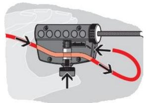
Push down on the thumb screw and feedthrough the rope to adjust the length of rope required. When the desired tension is reached, lock the rope into place by screwing in tight the thumb screw. Cut off excess rope and terminate the end inside the tensioner as shown.
