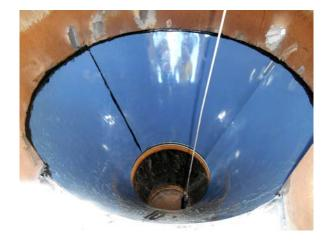
The K-Slip® Rubber Backed UHMWPE Flow Liner features a low co-efficient of friction polyethylene lining material, with a synthetic rubber backing (SBR). The thin flexible nature of Kinder Australia's K-Slip® Rubber Backed UHMWPE Flow Liner allows almost any complicated shape to be lined including bins, hoppers, and chutes, providing a uniform and therefore controlled rate of flow. The installation to a metal surface is by normal cold rubber bonding.
