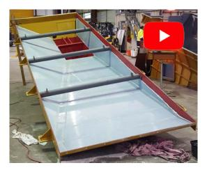
Round corners and acute angles do not fix well with fasteners; in fact, they often provide another point on which the material can bridge.
