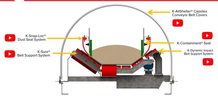
The effective suppression of dust particles around high pressure and poorly designed conveyor transfer points can be achieved by installing <a href="https://example.com/stalling">The Essential SNAP Seal</a> – Dust Containment Combination.
