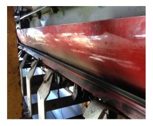
Finally, "The Essential SNAP Seal" incorporates K-AllShelter® Capotex Conveyor Belt Covers, a protective barrier, aiding airborne dust reduction and protection from extreme environmental elements. These covers also help to control moisture levels of conveyed materials, further controlling dust emissions.
