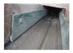
The K-Containment® Seal enhances the success of the outer seal by reducing the high internal pressure experienced inside the chute and protects the vulnerable chute edges from damage.
