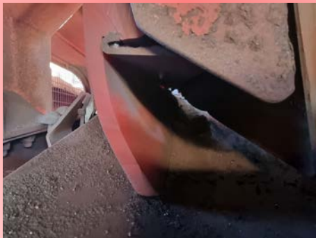
AFTER PHOTOS: Kinder The Essential SNAP Seal - Dust Containment after installation.
