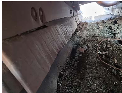
BEFORE PHOTOS: Duo plate hard/rubber skirting prior to Kinder's dust solution installation.
