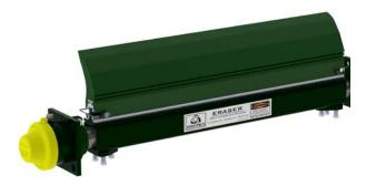
Designed to handle the most demanding applications with ease and efficiency, this proven effective belt cleaning system is equipped with a **184mm tall** polyurethane blade. It's also designed to handle most conveyor cleaning with 6mm thick, 76mm x 76mm powder-coated tube stock steel maintenance and corrosion-resistant, galvanised Schedule 80 pipe stub ends for superior strength and durability.
