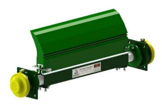
Built for high speed, high tonnage belt applications, this belt cleaning system delivers an extremely effective cleaning performance from the **305mm** polyurethane Raptor blade and rugged 6mm, 89mm x 89mm box steel mainframe. Suitable for use on conveyors with large head pulleys, big loads and the harshest mining applications
