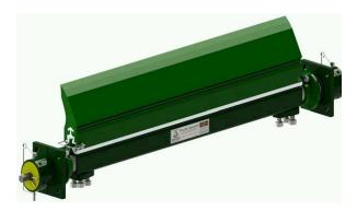
Lightweight in design, reliable, powerful and proven cleaning performance to match, this belt cleaning system is ideally suited for portable equipment with tight clearance restrictions. The system has a very compact mounting footprint with only a 114mm protrusion from the mounting structure and a highly effective cleaning performance delivered by the 152mm tall polyurethane blade.
