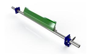
Ideally suited for pit and quarry applications, this cost-effective belt cleaning system is designed for performance and reliability. The system features a simple, effective and easy to install spring tensioning unit and the 152mm tall polyurethane blade utilised requires minimal to no maintenance.
