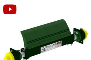
Design with superior strength and durability in mind, this belt cleaning system is suitable for use on conveyors with crowned head pulleys and to withstand heavy vibrations. The system incorporates a reinforced mainframe and a heavy- duty channel attachment design. The effective cleaning performance is delivered by the systems heavy duty 178mm tall polyurethane blade.
