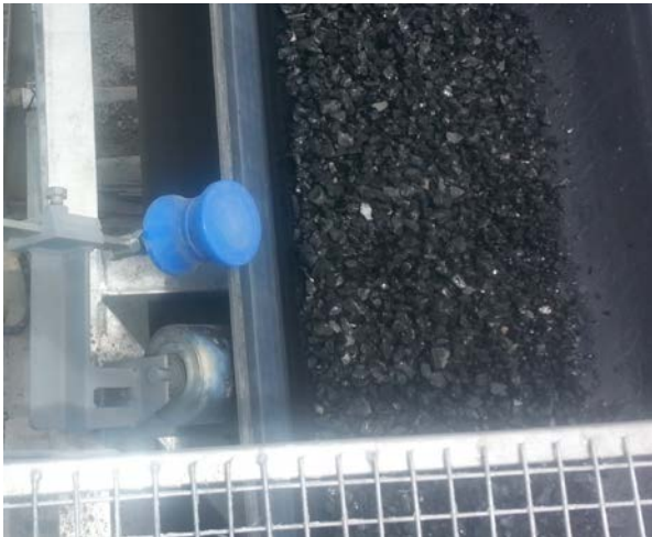
LEFT K-HD Polyurethane Side Guide Roller Installation
