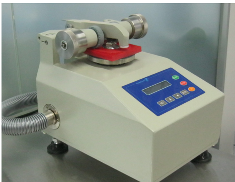
Photo: Taber Abrasion testing a specimen of K-Superline® under weighted abrasive wheels. The Abrasion Resistance is calculated as loss in weight per abrasion cycle.
