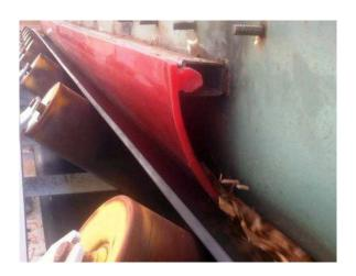
Because of the low coefficient of friction there is a power saving by producing 60% less drag on the conveyor belt than traditional skirting rubber.
