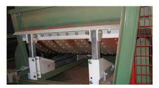
K-Flexal® Elastic Belt Support System consists of cross belt polyurethane elastic straps, with its flexibility and elongation design feature allowing better absorption of energy and even weight dispersion of the conveyed bulk material.
