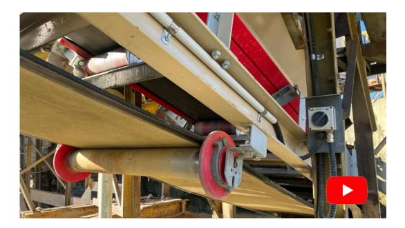
The <u>K-Commander® Tracking Discs</u> are a highperformance economical means to track and align a wandering conveyor belt, which is suitable for most installations and bulk materials handling applications.
