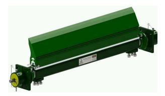
Lightweight in design, reliable, powerful and proven cleaning performance to match, this belt cleaning system is ideally suited for portable equipment with tight clearance restrictions. The system has a very compact mounting footprint with only a 114mm protrusion from the mounting structure and a highly effective cleaning performance delivered by the 152mm tall polyurethane blade.
