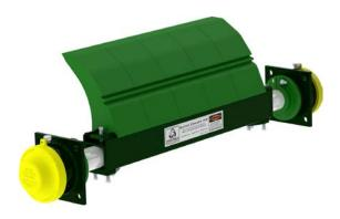
Designed for extreme strength and durability this belt cleaning system utilises segmented blade technology, large **269mm tall polyurethane blade** and 6mm thick, 89mm x 89mm tube stock steel mainframe and corrosion-resistant, galvanised Schedule 160 pipe stub ends to handle the harshest environments. Ideally used for conveyors with large crowned head pulleys, big loads, harsh conditions and/or fast belt speeds.
