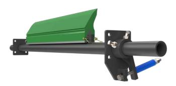
Ideally suited for pit and quarry applications, this cost-effective belt cleaning system is designed for performance and reliability. The system features a simple, effective and easy to install spring tensioning unit and the 152mm tall polyurethane blade utilised requires minimal to no maintenance.
