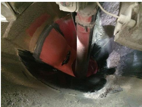
Above: Photo showing the worn ceramic lining trialled inside the wok. Below: photo of worn rubber lining
