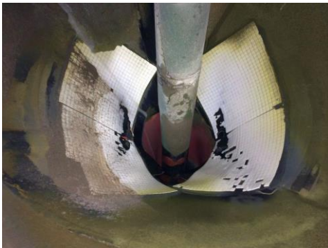
Above: Photo showing the worn ceramic lining trialled inside the wok. Below: photo of worn rubber lining
