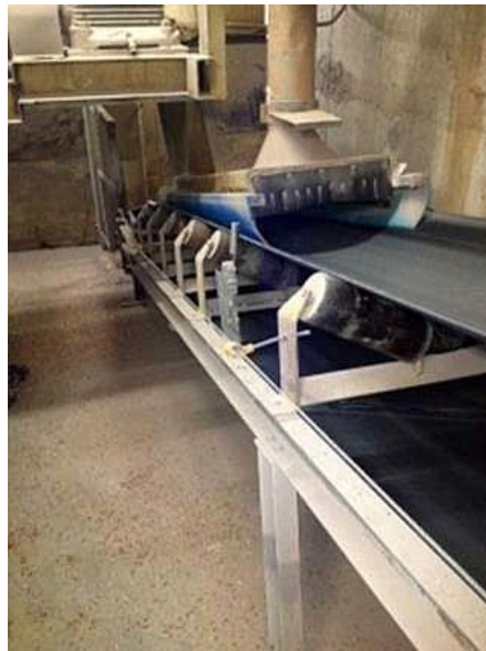
Photos of K-Snap-Loc® installed around the transfer point - the blue polyurethane indicates the Fire Resistant Anti Static FRAS properties.
