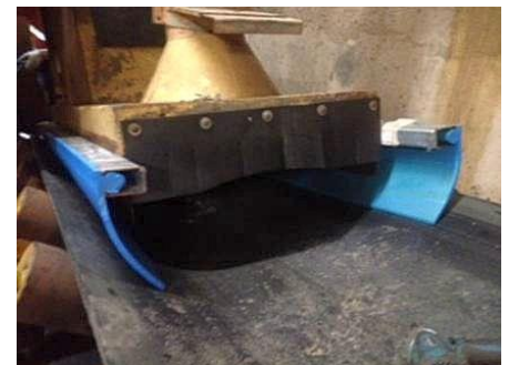
Photos of K-Snap-Loc® installed around the transfer point - the blue polyurethane indicates the Fire Resistant Anti Static FRAS properties.
