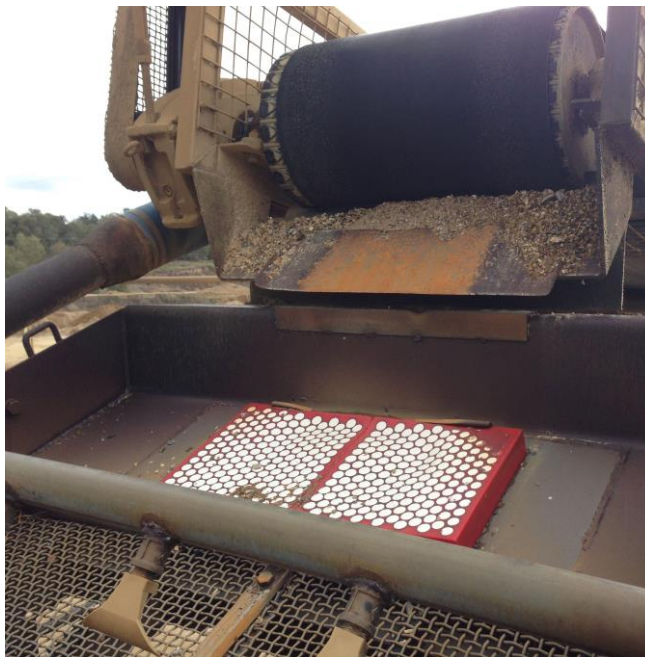
2013 photo of K-Redi-Liner ® Ceramic Lining still in place after 2 years and 4 months constant use
