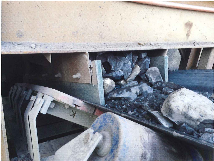
K-Containment Seal and K-Sure Belt Support System.
